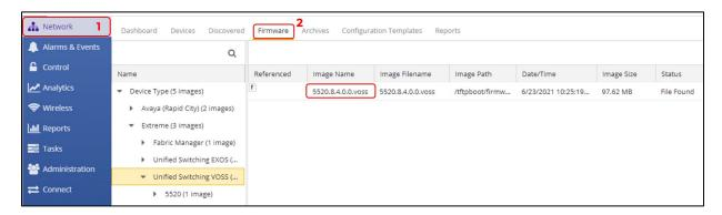
Copy and paste the desired image name. Note that the workflow uses FTP to transfer the image, and so the image must be located in /tftpboot/firmware/images.
