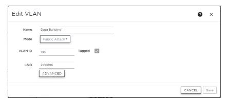
Confirm by inspecting the Fabric Attach assignments on the switch using the CLI command show fa assignment.
