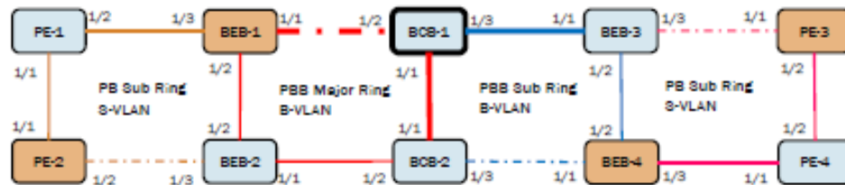
FIGURE 180 PBB interconnection node (BCB)
