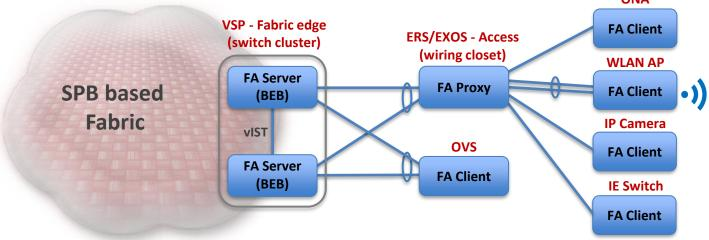
MLT LAG or LACP links between any FA element is supported, as long as each interconnection is a single logical link. Switch clustered FA Servers are only supported on VSP platforms.
