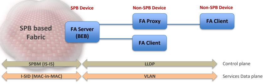
The two signaling planes are shown to illustrate which parts of the network are controlled by which protocols and what the "services" are delivered on. IE: Non-SPB/fabric devices only support VLANs for services.
