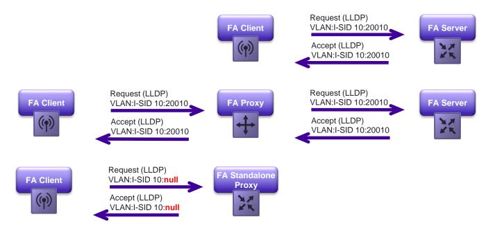
FA Standalone Proxy is a mode where the FA Proxy switch operates without the presence of an FA Server. This mode is only useful in situations
