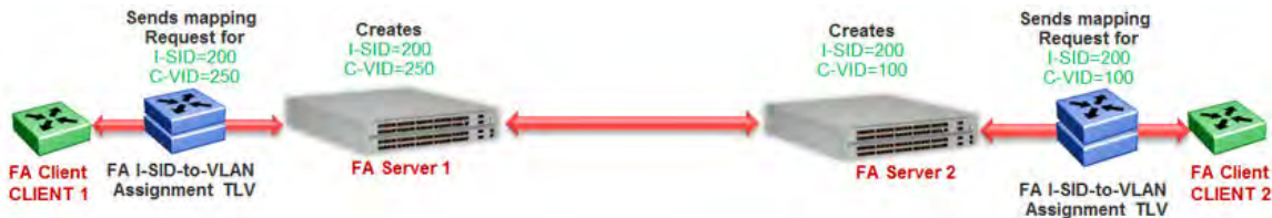
Figure 18: Learning of I-SID-to-VLAN mappings
