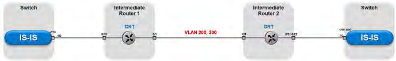
Figure 34: FE over Pseudowire traffic flow component view
